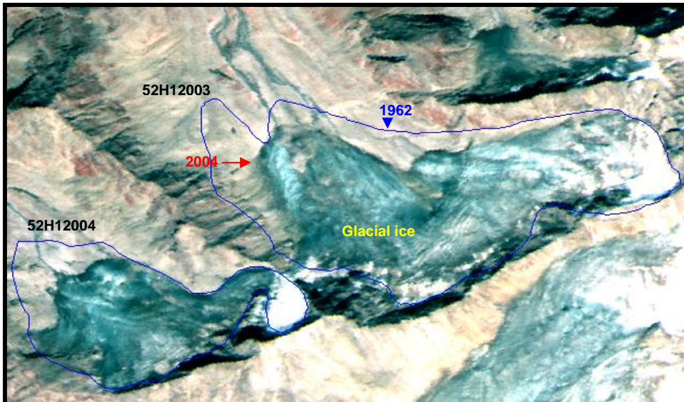
Fig. 2 A satellite imagery of glacier number 52H12003 and 52H12004 of LISS-IV sensor showing glacial boundary of 1962 and 2004. These are small mountain glaciers, showing negligible accumulation area. Maximum altitude of these glaciers is around 5200 m. This is very close to snow line at the end of ablation season and such glaciers are expected to experience terminal retreat.
